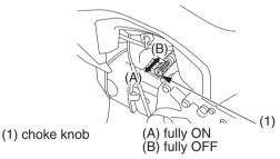
1. Pull the choke knob (1) out all the way to fully ON (A).
