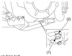
(1) oil drain bolt(2) sealing washer
