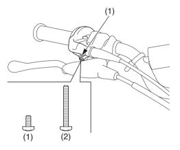
(1) M5x10 screw (2) M5x40 screw You can reduce throttle grip movement.
