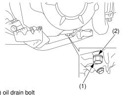
(1) oil drain bolt(2) sealing washer
