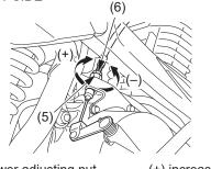
(5) lower adjusting nut(6) lower lock nut
