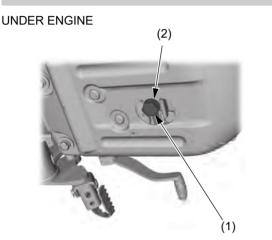
(1) oil drain bolt(2) sealing washer
