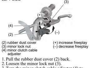
3. Turn the minor clutch cable adjuster (4) to obtain the specified freeplay.
