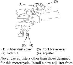
the lever side with the lock nut under the head of the adjuster.
