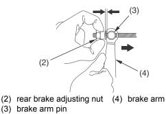
After adjustment, confirm the freeplay of the brake pedal.
