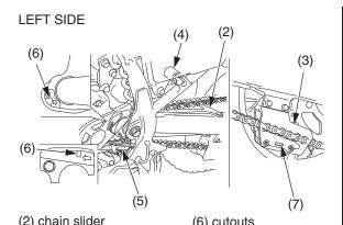
5. Replace the drive chain if chain slack is excessive when the rear axle is moved to the farthest limit of adjustment. Excessive slack indicates the chain is worn beyond its service limit.
