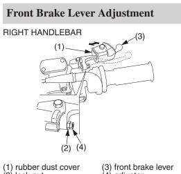
(2) lock nut (4) adjuster Never use adjusters other than those designed for this motorcycle. Install a new adjuster from
