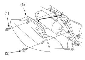
(1) seat mounting bolt(2) side cover bolt
