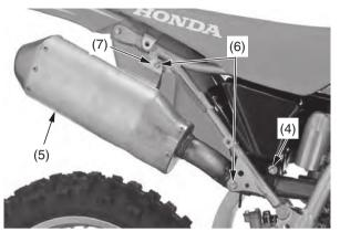
(4) muffler clamp bolt(5) muffler(6) muffler mounting bolts(7) washer
