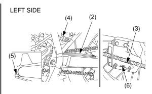
(2) chain slider(3) chain guide slider(4) chain roller
