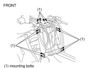
2. Check the security of all handlebar and fork mounting bolts (1). If any front suspension components appear worn or damaged, see your dealer for further inspection.
