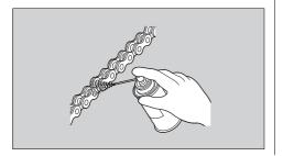
Do not use a steam cleaner, a high pressure cleaner, a wire brush, volatile solvent such as petrol and benzene, abrasive cleaner, chain cleaner or lubricant NOT designed specifically for O-ring chains as these can damage the rubber O-ring seals.
