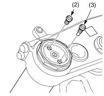
(2) pressure release screw A(3) pressure release screw B
