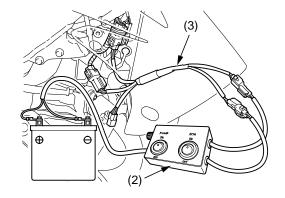
(2) battery harness(3) battery harness adapter
