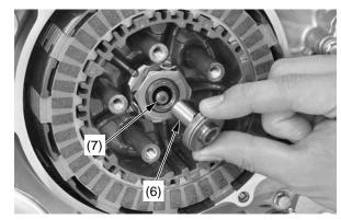
(6) clutch lifter(7) clutch lifter rod
