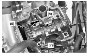
(7) left camshaft bearing(8) camshaft(9) cam chain
