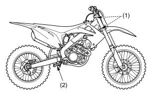
(1) steering head bearings(2) suspension pivot points
