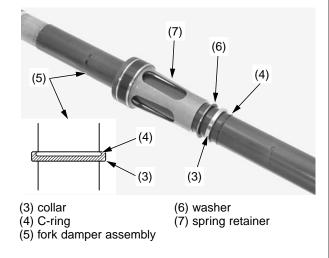
4. Blow out the oil completely off the fork spring (8) using compressed air. Install the fork spring to the fork damper assembly (5). Install the fork damper assembly to the fork
