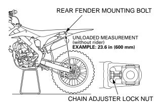
3. Measure the *loaded with rider* dimension. Remove the workstand. With two helpers available, sit as far forward as possible on your CRF's seat, wearing your riding apparel. Ask one helper to steady your CRF perfectly upright so you can put both feet on the pegs. Bounce your weight on the seat a couple of times to help the suspension overcome any situation and settle to a good reference point.
