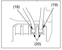
(18) red wire terminal(19) black wire terminal(20) fuel pump base terminals(21) O-ring (new)(22) fuel pump unit
