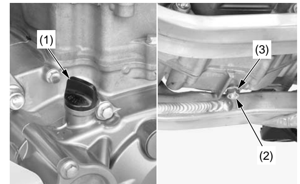
(1) engine oil fill cap/dipstick (2) engine oil drain bolt (3) sealing washer (new)
