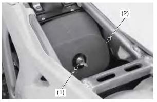
(1) air cleaner retaining bolt(2) air cleaner assembly
