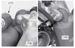
(17) rear shock absorber(19) nut(18) rear shock absorber upper bolt
