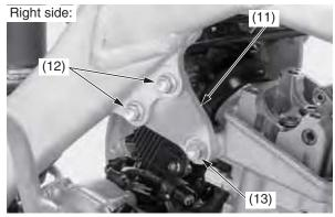
(10) left cylinder head hanger plate (11) right cylinder head hanger plate
