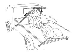
To secure your CRF, brace the front wheel against the front of the truck bed or trailer rail. Attach the lower ends of two straps to the tie-down hooks on truck bed or trailer rail. Attach the upper ends of the straps to the handlebar (one on the right side, the other on the left), close to the fork.
