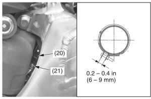
(20) air cleaner connecting tube(21) air cleaner connecting tube band screw
