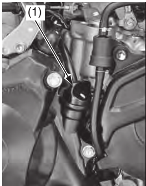
(1) engine oil fill cap/dipstick (2) upper level mark (3) lower level mark
