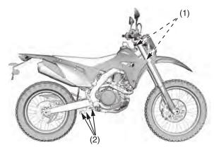
(1) steering head bearings(2) suspension pivot points
