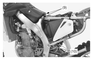
(9) subframe upper mounting bolts (10) subframe lower mounting bolts
