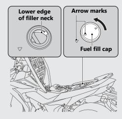
Do not fill with fuel above the lower edge of the filler neck.
