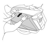
To close the saddlebags, place your hands flat on the edges of its lid and press down until it is firmly closed and check the saddlebags open indicator is not displayed.
