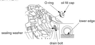
Change the oil with the final drive at normal operating temperature to assure complete and rapid draining.
