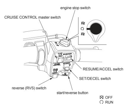
The engine stop switch is used to stop the engine in an emergency. To operate, turn the switch to the OFF position. The switch must be in the RUN position to start the engine, and it should normally remain in the RUN position even when the engine is OFF.
