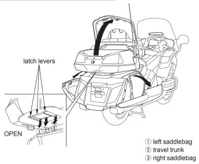
To open the travel trunk, pull the middle latch lever down.
