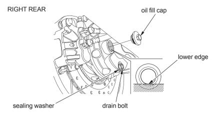
Change the oil with the final drive at normal operating temperature to assure complete and rapid draining.
