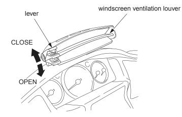
You can adjust the windscreen ventilation louver with the lever to control and direct the flow of fresh air.
