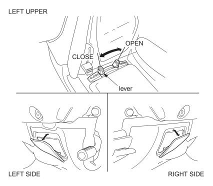
You can adjust the foot warmer ventilation louvers with the lever to control and direct the flow of warm air.
