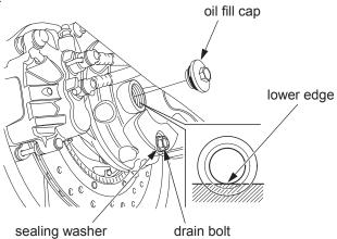
Change the oil with the final drive at normal operating temperature to assure complete and rapid draining.
