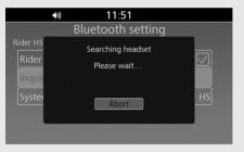
The names of the devices detected are displayed on the background screen. Press or ENT switch to exit the search mode.
