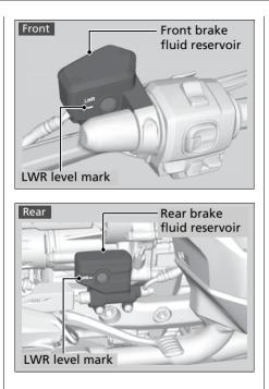
If the brake fluid level in either reservoir is below the LWR mark or the brake lever and pedal freeplay becomes excessive, inspect the brake pads for wear. If the brake pads are not worn, you most likely have a leak. Have your vehicle inspected by your dealer.
