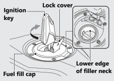
Do not fill with fuel above the lower edge of the filler neck.
