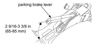
If adjustment is necessary, have the parking brake adjusted by your Honda dealer.
