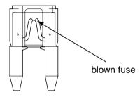
Check all the fuses before looking elsewhere for another possible cause of the problem. Replace any blown fuses and check component operation.
