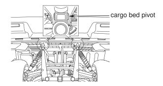
Lubricate the cargo bed latch pivots as shown in the following illustration.
