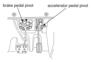
Lubricate the parking brake pivot as shown in the following illustration. Remove the center panel (page 130).
