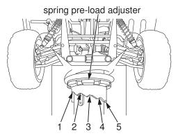
The spring pre-load adjuster has 5 positions for different load or riding conditions. Before adjusting the spring pre-load, jack up your Honda MUV (page 94) to avoid damaging the adjusters.
