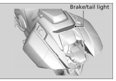
The brake and tail light uses several LEDs. If there is a LED which is not turned on, see your dealer for servicing.
