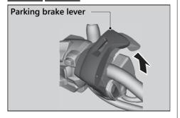
Place your motorcycle on a firm, level surface. Stop the engine and push your motorcycle while set the parking brake to check the efficacy of the parking brake.
